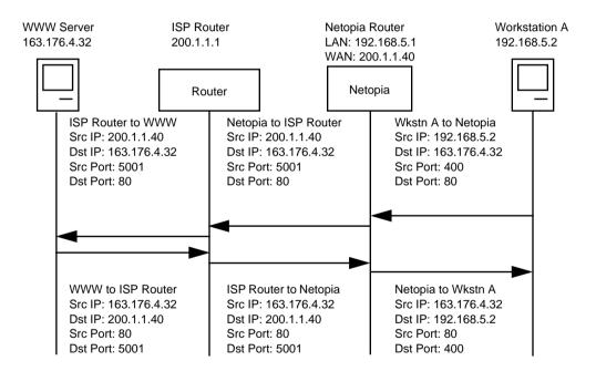
As you can see, the IP packet from Workstation A is sent to the Netopia R5000 Series Router, the source IP address is substituted with 200.1.1.40 and the source port is substituted with 5001, then the IP packet checksum is recalculated. When this modified packet reaches the WWW server on the Internet, the WWW server responds and sends the IP packet back to destination IP address 200.1.1.40 and destination port 5001.
